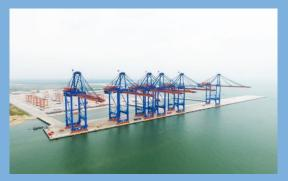
Each crane is 93m high, 150m long, 27m wide, weighs more than 1,700 tons, has a reach of 70m, equivalent to 24+2 container rows, and is capable of handling container cargo of up to 65 tons from vessels up to 200,000 DWT.
